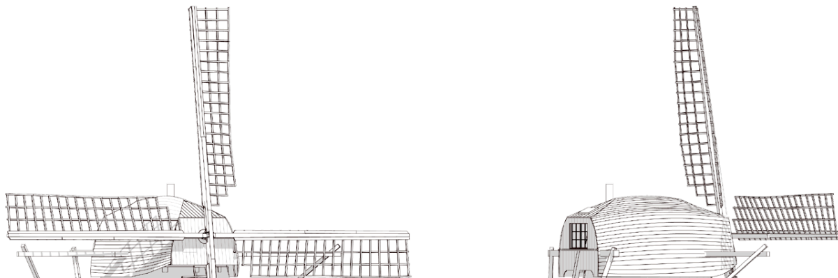
11. Renovation project for Habicht dutch type windmill in Järvamaa, Estonian mainland, 2008. This 5-story windmill, built in 1894, was until 2008 an empty stonecone. The owner, who bought the empty cone, wanted to have a summer cottage inside, built into a traditional-looking windmill. The exterior is made as authentic as possible, and the cap is almost real - when needed, it only needs a crane to remove the cap, change the curb ring to make the cap rotating, and place back the same cap, then the exterior is ready for grinding. Offcourse in this case the windmill needs mechanisms inside, but right now (2008) the mill is under construction and will soon be an interesting summer house.
